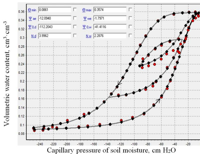
Figure 2. Identification of the parameters of the model proposed by the authors of the article, by fit-approximating of the measured WRC data on the main branches; prediction of the primary wetting branch, the secondary drying branch, the tertiary wetting branch of the WRC hysteresis loop of the white silica sand [1].
