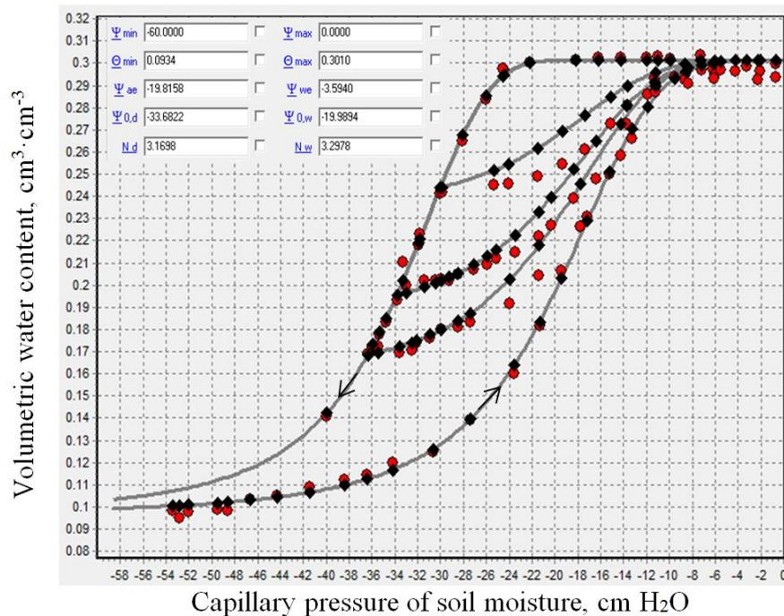
Figure 3. Identification the parameters of the model proposed in this paper by fit-approximating the measured data on the WRC main branches. Predicting for three primary wetting branches of the hysteresis loop of the dune sand [2].
