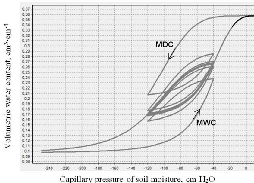
Figure 1. Sequence of the drying and wetting branches of the WRC hysteresis loop of the white silica sand [1] under oscillation of capillary pressure in a fixed range.
